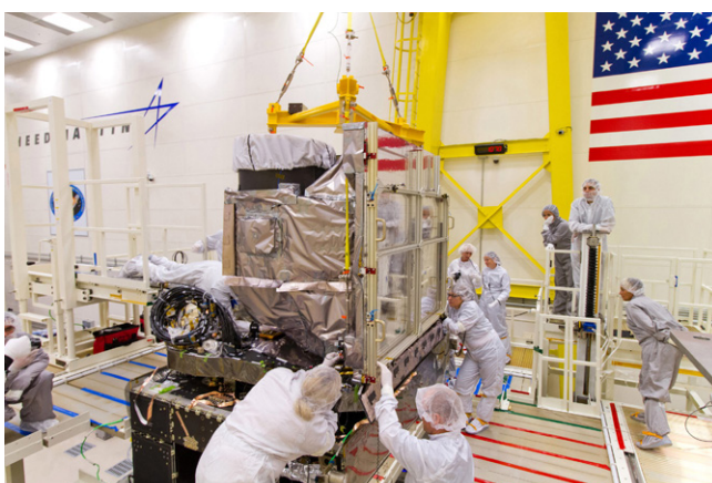
Installation of the GOES-R ABI onto the spacecraft. Credit: Lockheed Martin
